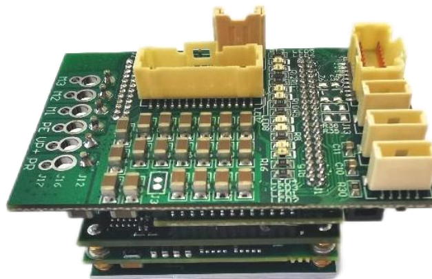
Power Connection (recommended for >15A Output Current, but optional for ≤ 15A)
