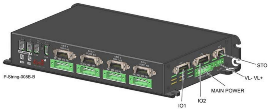
Figure 3: IO, Power, Control Power and STO Connector Locations
